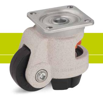
**Brackets:** HRP/HRSP series - Made of die-cast aluminium, with sealed ball bearing in the swivel head, steel top plate fitting.
