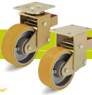
Wheels: GTH series - Tread: Made of high-quality polyurethane-elastomer Blickle Extrathane®, 92° shore A, light brown, non-marking, non-staining. Wheel centre: Made of rugged grey cast iron, with grease nipple, lacquered, silver.
