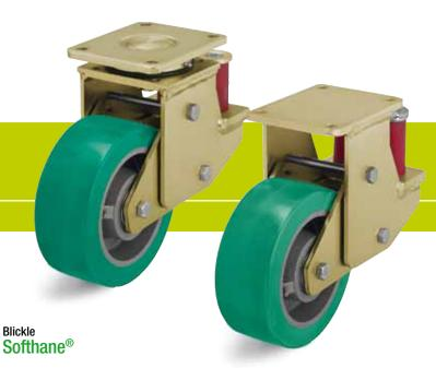
Wheels: GST series - Tread: Made of high-quality polyurethane-elastomer Blickle Softhane®, 75° shore A, green, non-marking, non-staining. Wheel centre: Made of rugged grey cast iron, with grease nipple, lacquered, silver.
