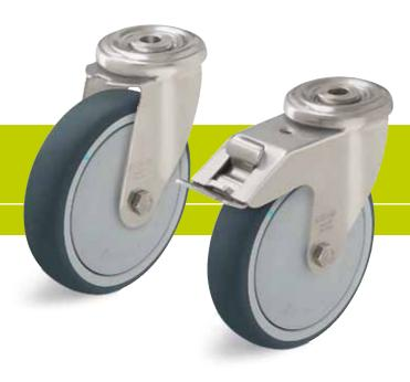
**Wheels:** PATH series - Tread: Made of high-quality thermoplastic polyurethane, 94° shore A, dark grey, non-marking, non-staining.
