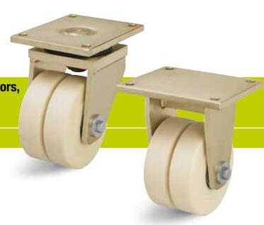
Wheels: GSPO series - Made of high-quality, impactresistant, hard and tough, highly compressed cast nylon,  $80^{\circ}$  shore D, natural beige. Bearing type: Two pressed-in ball bearings.
