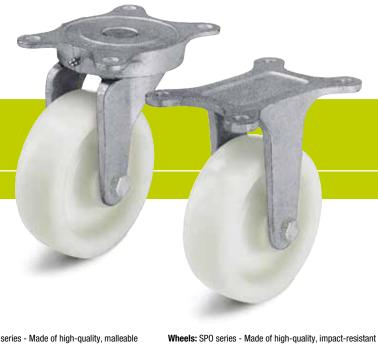
Brackets: LT/BT series - Made of high-quality, malleable cast iron, swivel bracket with double ball bearing in the swivel head (wheel Ø 75 mm: single ball bearing), ball protection by the special top plate and fork design, fitted grease nipple.
