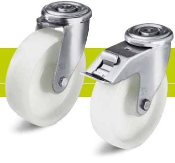
$\mbox{\bf Brackets:}$  LER series - Made of pressed steel, with double balk bearing in the swivel head, strong central kingpin, ball protection by the special top plate and ball disc design. The special Blickle dynamic riveting process of the swivel head results in minimal swivel head play and smooth rolling characteristics with an increased service life achieved by the work hardening of the ball race grooves. Bolted wheel axle.
