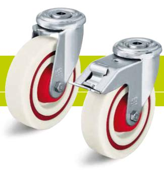
Wheels: POW series - Made of high-quality, impactresistant nylon, 70° shore D, white, with elastic solid rubber  $damping\ ring, red.$
