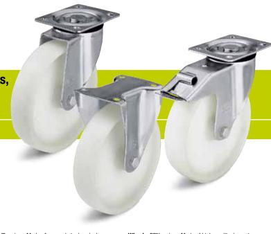
**Wheels:** PPN series - Made of high-quality, impactresistant polypropylene, 60° shore D, natural white. Bearing types: Plain bore or roller bearing. Detailed description: Page 293 and 49
