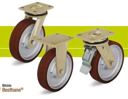
Brackets: LS/BS series - Particularly rugged welded steel construction, swivel bracket with axial grooved ball bearing DIN 711 and tapered roller bearing DIN 720 in the swivel head, dust and splash-proof, fitted grease nipple, bolted and secured with a welded very strong central kingpin. Bolted wheel axle.
