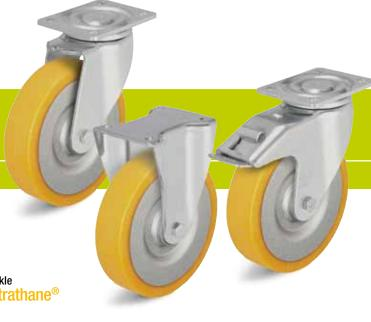
Wheels: SETH series - Tread: Made of high-quality polyurethane-elastomer Blickle Extrathane®, 92° shore A, light brown, non-marking, non-staining. Wheel centre: Made of pressed steel, with tubular steel hub, lacquered, silver.
