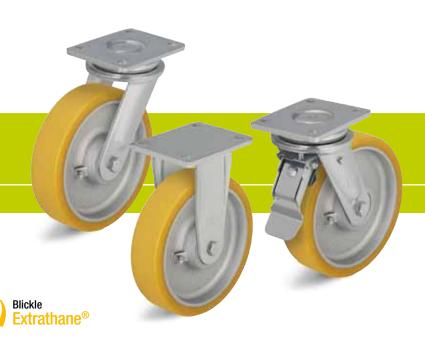
Wheels: GTH series - Tread: Made of high-quality polyurethane-elastomer Blickle Extrathane®, 92° shore A, light brown, non-marking, non-staining.
