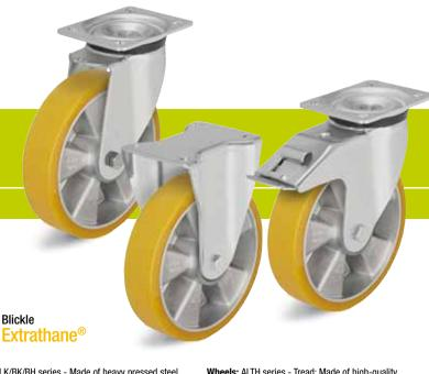
Wheels: ALTH series - Tread: Made of high-quality polyurethane-elastomer Blickle Extrathane®, 92° shore A, light brown, non-marking, non-staining. Wheel centre: Made of die-cast aluminium. Bearing type: Two pressed-in ball bearings. Detailed description: Page 246 and 48
