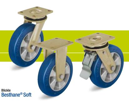
Wheels: ALBS series - Tread: Made of high-quality polyurethane-elastomer Blickle Besthane® Soft, 75° shore A, very low rolling resistance, high dynamic load capacity, blue, non-marking, non-staining. Wheel centre: Made of die-cast aluminium. Bearing type: Two pressed-in ball bearings. Detailed description: Page 238 and 47
