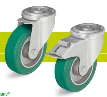
Wheels: ALST series - Tread: Made of high-quality polyurethane-elastomer Blickle Softhane®, 75° shore A, green, non-marking, non-staining. Wheel centre: Made of die-cast aluminium. Bearing type: Two pressed-in ball bearings. Detailed description: Page 222 and 47
