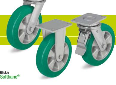
Wheels: ALST series - Tread: Made of high-quality polyurethane-elastomer Blickle Softhane®, 75° shore A, green, non-marking, non-staining. Wheel centre: Made of die-cast aluminium. Bearing type: Two pressed-in ball bearings. Detailed description: Page 222 and 47
