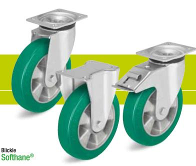
Wheels: ALST series - Tread: Made of high-quality polyurethane-elastomer Blickle Softhane®, 75° shore A, green, non-marking, non-staining. Wheel centre: Made of die-cast aluminium Bearing type: Two pressed-in ball bearings.
