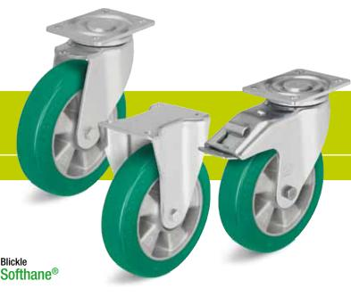
Wheels: ALST series - Tread: Made of high-quality polyurethane-elastomer Blickle Softhane®, 75° shore A, green, non-marking, non-staining. Wheel centre: Made of die-cast aluminium. Bearing type: Two pressed-in ball bearings. Detailed description: Page 222 and 47
