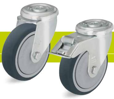
Wheels: PATH series - Tread: Made of high-quality thermoplastic polyurethane,  $94^{\circ}$  shore A, dark grey, non-marking, non-staining.
