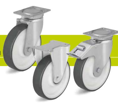
Wheels: POTH series - Tread: Made of high-quality thermoplastic polyurethane, 94° shore A, dark grey, non-marking, non-staining.
