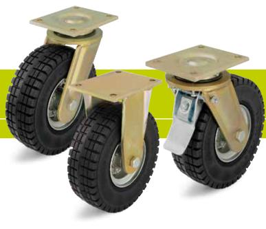
Wheels: VLE series - Tyres: With hard rubber core, black. Wheel Ø 250-306 mm: 2-component tyres, super-elastic, abrasion-resistant tread. Wheel Ø 405-525 mm: 3-component tyres, super-elastic cushion layer, abrasion-resistant tread. Rims: Made of heavy pressed steel, bolted (flat based rim), with tubular steel hub or reinforced rim version, zinc-plated, blue-passivated, Cr6-free. Bearing type: Two pressed-in ball bearings. Detailed description: Page 202 and 46
