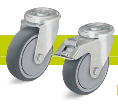
Brackets: LER series - Made of pressed steel, with double ball bearing in the swivel head, strong central kingpin, ball protection by the special top plate and ball disc design. The special Blickle dynamic riveting process of the swivel head results in minimal swivel head play and smooth rolling characteristics with an increased service life achieved by the work hardening of the ball race grooves.
