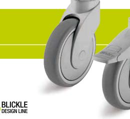
Brackets: LWG series - Made of high-quality, impactresistant and reinforced nylon, with encapsulated, double-sealed grooved ball bearing in the swivel head, with zinc-plated, blue-passivated bolted and secured steel plug-in stem fitting (Cr6-free), silver grey RAL 7001.
