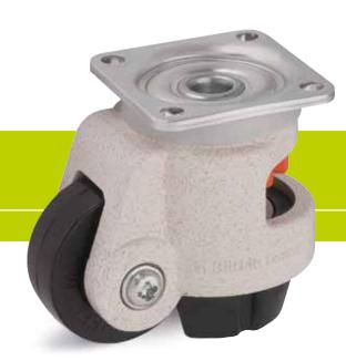
Brackets: HRP/HRSP series - Made of die-cast aluminium, with sealed ball bearing in the swivel head, steel top plate fitting.
